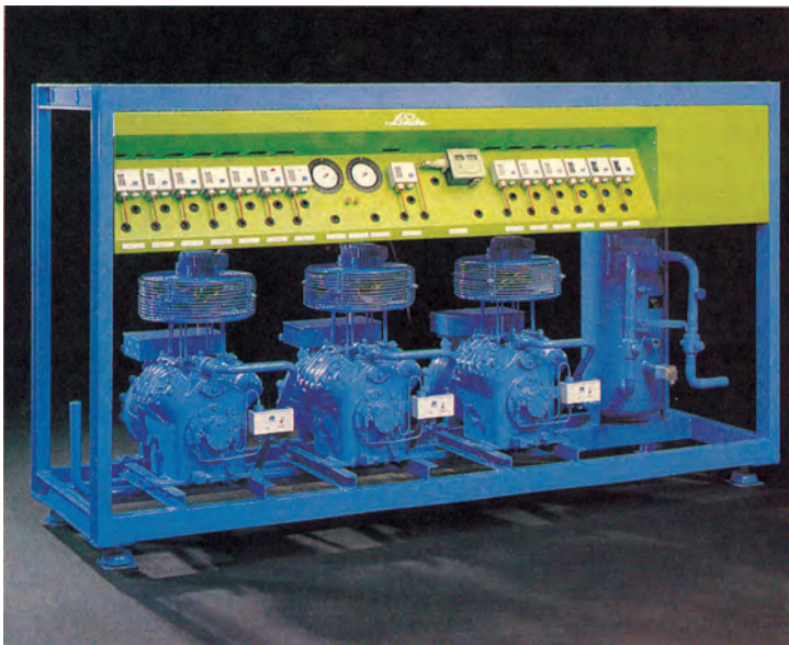
Commercial multi-compressor refrigeration system installed in a supermarket
