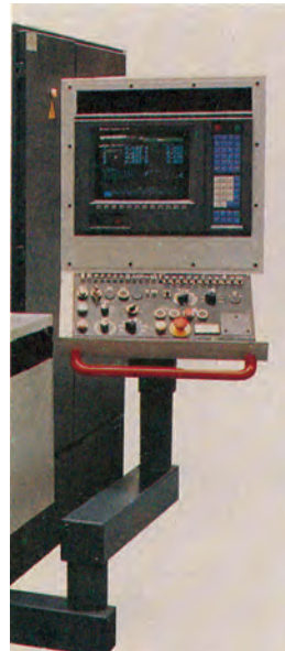
Machine control unit (MCU)
