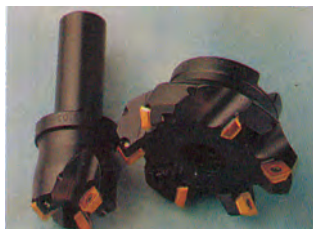
Cutting heads with inserts
