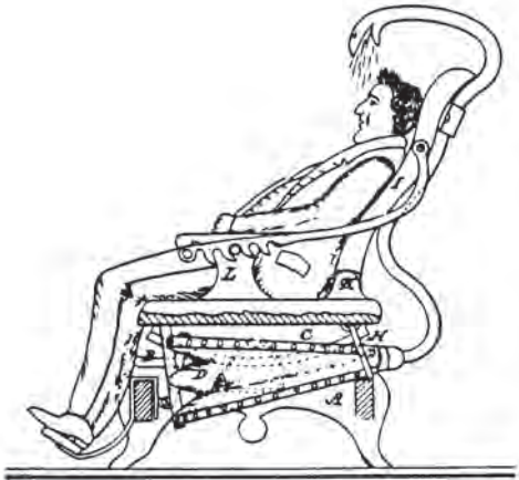
Rocking motion operates bellows
