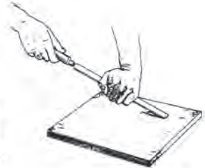
7. Scraping metal surfaces
