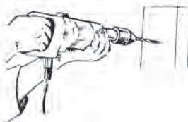
15. Cutting holes in metal pieces (drilling)
