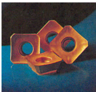
Inserts, the modern CNC cutting tools
