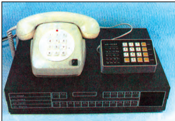
electronic telephone switchboard
