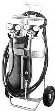
Cylinders with oxygen and acetylene
