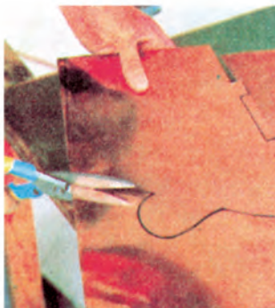
15 Shearing thin sheets of metal
