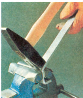
10 Bending metal sheets
