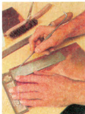
4 Scribing lines or circles on metal surfaces
