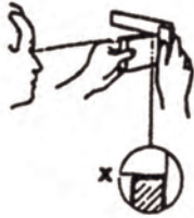
20 Checking right angles
